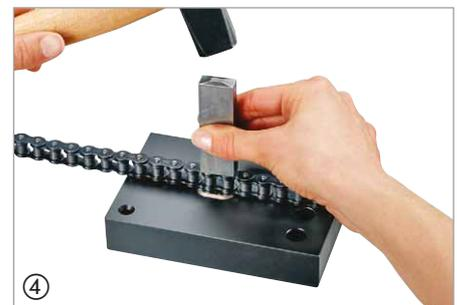
A new outer link plate is fitted using fetching-up punch (C) ④. With parallel bearing pin chain it is possible to over fit the outer link plate on the bearing pins. It is necessary to check that the joint remains free and easily moveable after fitting.
