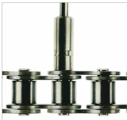
The new adapter is set onto the extended pin. Seize it with the gripping jaws ② and clamp it with the tool. Thus repaired, the chain is operational again.
