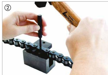
The fork (A 1) is placed through the chain at the outer link which is to be removed. The fork is then supported by the anvil and the bearing pins are driven through the chain using punch (B) ②. Multiple strand chains can also be broken in this way, the fork should then be placed in the top strand of the chain.
