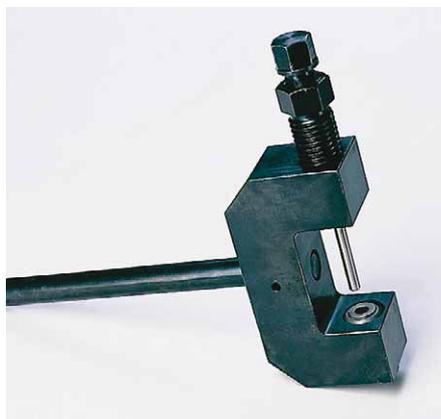
Tool for dismantling accumulation chain M 120 SF and M 127 SF with 3/4 inch pitch (available from stock)
