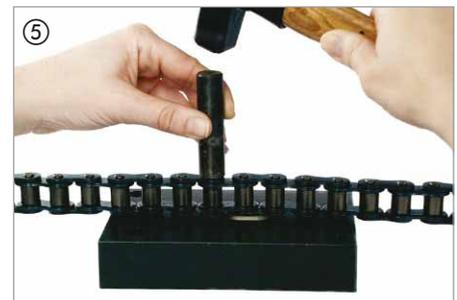
The newly fitted outer link then requires the bearing pin ends to be riveted. This is done with riveting punch (E) ⑤.
