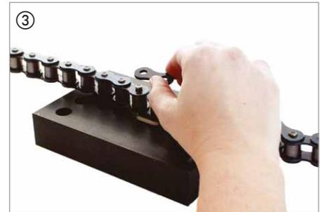
The procedure used is common to both shouldered and parallel bearing pin chains. The new riveting link connects the two inner links. This connecting link is supported by an insert in riveting plate (D) ③.
