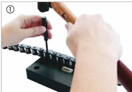
The outer link to be broken has to be placed over the holes in the riveting plate (D). The bearing pins are hammered flush with the outer plate and then driven through the chain with pin punch (B) whose diameter must be smaller than that of the bearing pin ①. To assist when breaking large pitch chains it is recommended that the rivet head is initially ground away.
