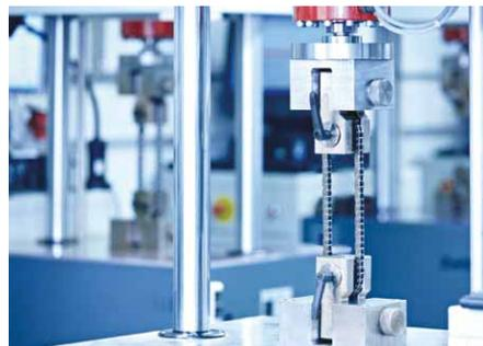
More than 25 pulser are available for testing dynamic fatigue strength according to different testing methods
