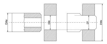
Interference fit shaft-hub connections can be achieved by cooling the shaft or heating the hub. This type of connection is not widely used for the following reasons:
