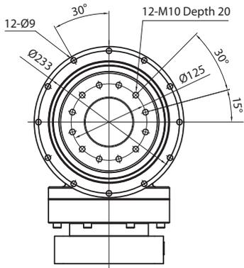
Input bore size  $\leq \text{Ø}38\text{mm}$
