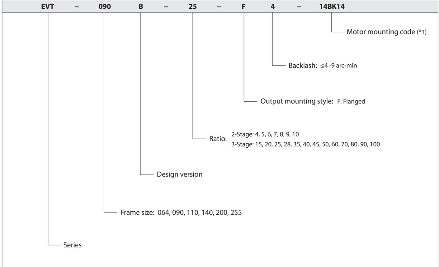
\*1) Motor mounting code varies depending on the motor. Use the selection tool link below to configure the code.
