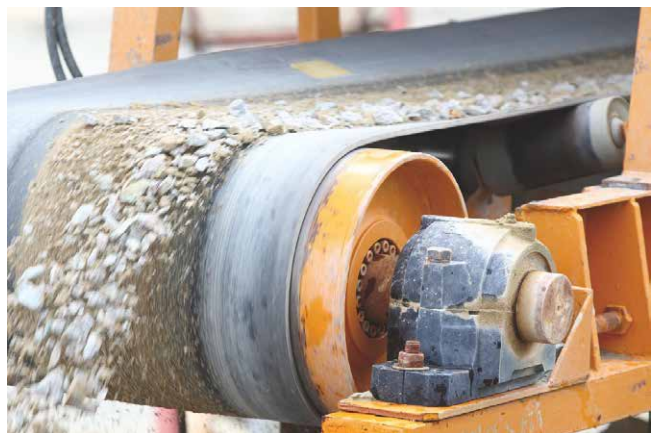
SIT-LOCK® 1 used for a conveyor belt pulley.
