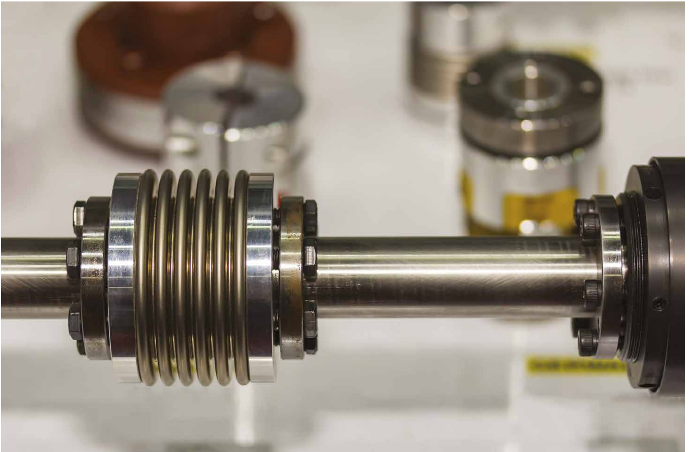
Locking a bellows coupling using SIT-LOCK® 16.
