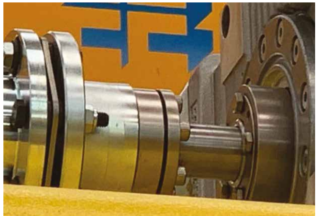
SIT-LOCK® 3 used for a disc coupling.
